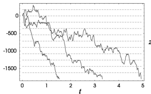
FIG. 5. Sample trajectories of particles moving through a ponderomotive ratchet potential depicted in Fig. 4 (arbitrary units). The location of individual barriers is shown by dashed lines ( \Delta L \gg L_1, L_2 ).
